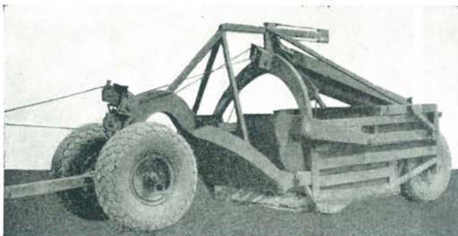
12-yard carryall with pan up and closed.
