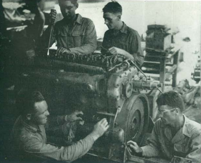
Tuning up a rebuilt Gray Marine Diesel in the 3d echelon shops of the 1461st.
