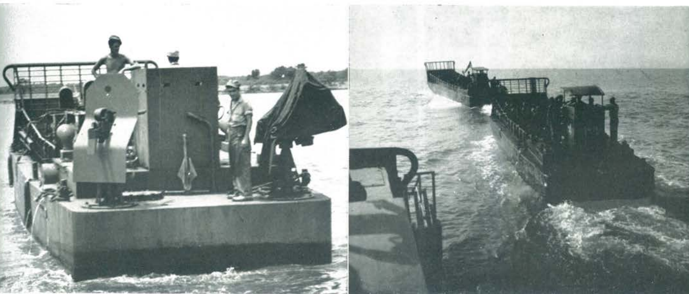
Left: LCM(3) showing Heintz mount without gun and Danforth-type anchor. Right: LCM(6)s viewed from deck of LCMG.
