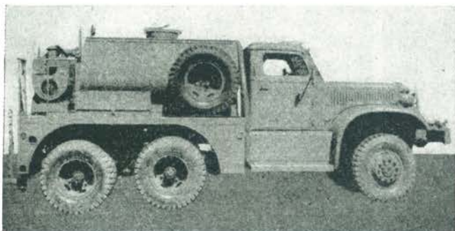
1000-gallon water distributor truck.
