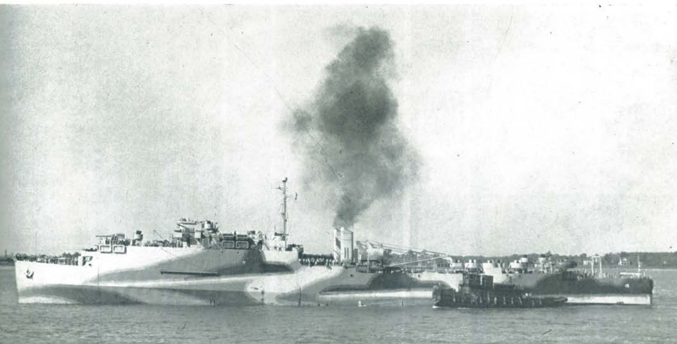
LSD — a high speed floating drydock for LCTs and LCMs.
