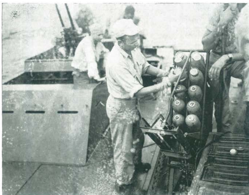
Turret of LCS(S) tied up alongside LCMG. Rockets on latter's MK VII launcher (magazine type) are being fused.
