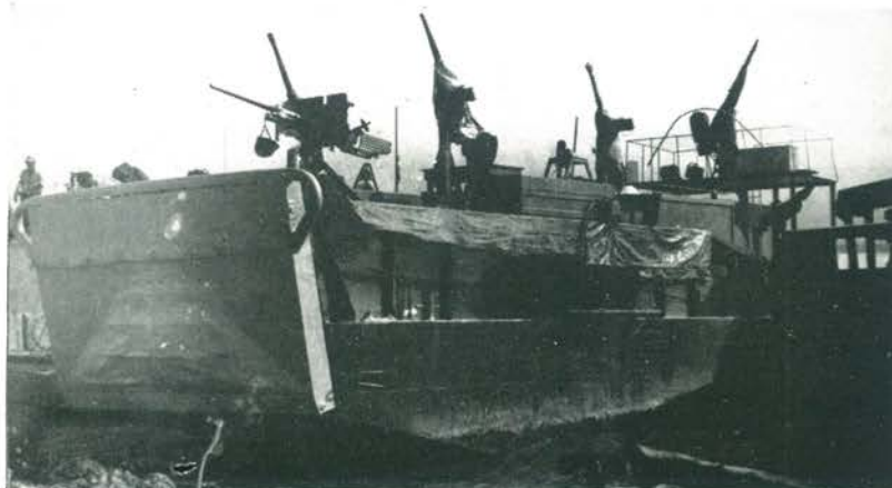
LCMG MB1 with 37 mm gun, 3 .50 calibre machine guns and 20 mm automatic cannon on flying bridge.
