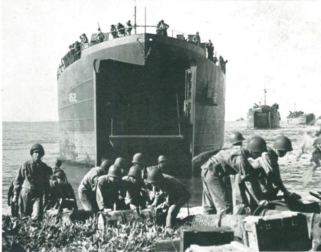
Bow views of LSTs showing doors and ramps.
