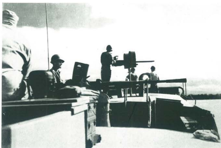
Looking forward on LCMG MCI; note the Jap 25 mm automatic cannon in the after cockpit.
