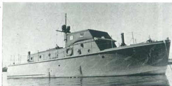
Type AC command boat developed for EAC by Gar Wood but never used overseas because of unreliable engine.
