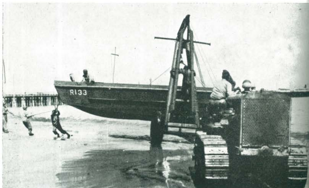
20-ton LeTourneau tractor-crane with LCPR in its clutches at Monterey.
