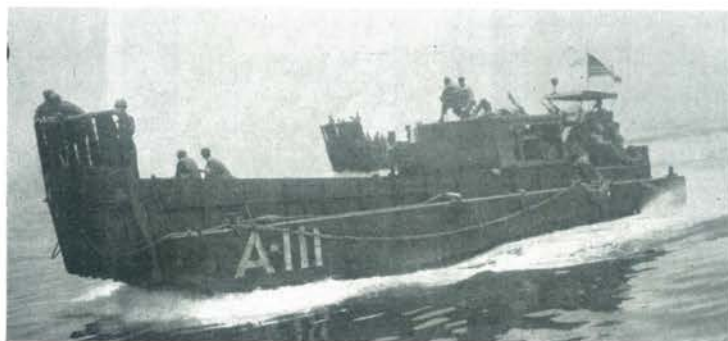
LCM(6) with removable cabin for crew of four.
