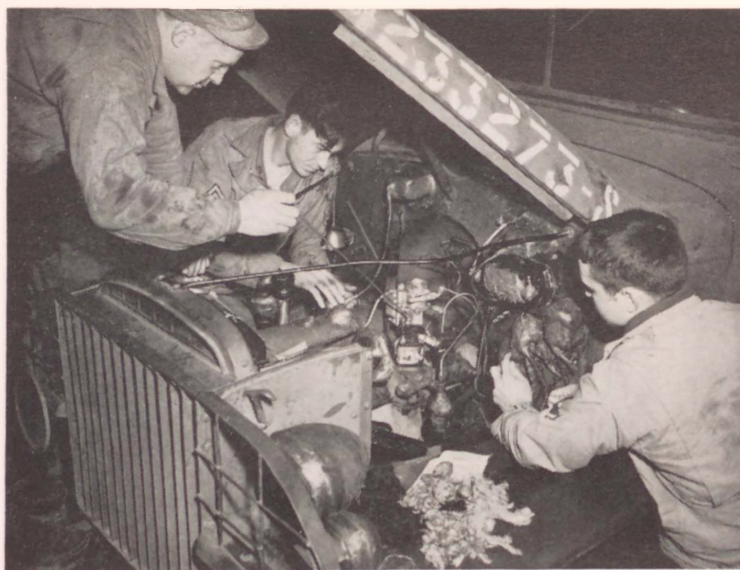
Motors were waterproofed
